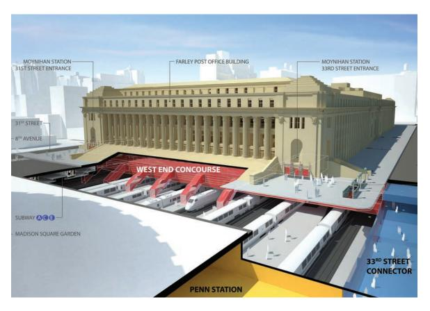
A cross section of improved platforms and new passenger access at Moynihan Station. Phase 2 of the project will allow Amtrak to relocate operations and passengers to Moynihan Station.
