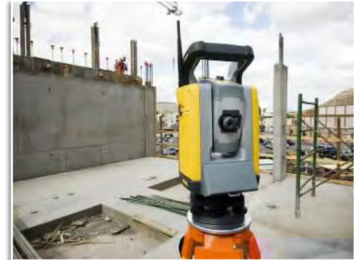
Total Station Used Directly in the Field
